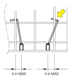
Hook always placed underneath rebar and secured with wire.
